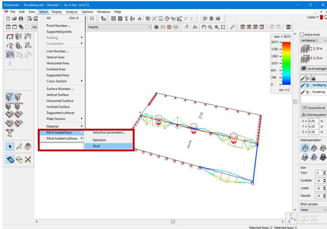
Note: the skull arises when more reinforcement is required than the maximum allowed amount imposed by the standard.
