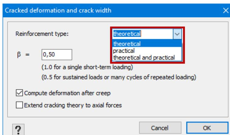
The option 'only practical reinforcement' is interesting when you need to recalculate the cracked deformation in an existing slab for example. Using the button
